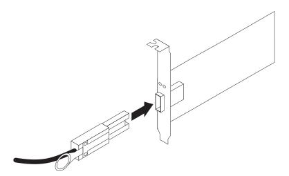
Figure 16. Connecting a mini-SAS cable
